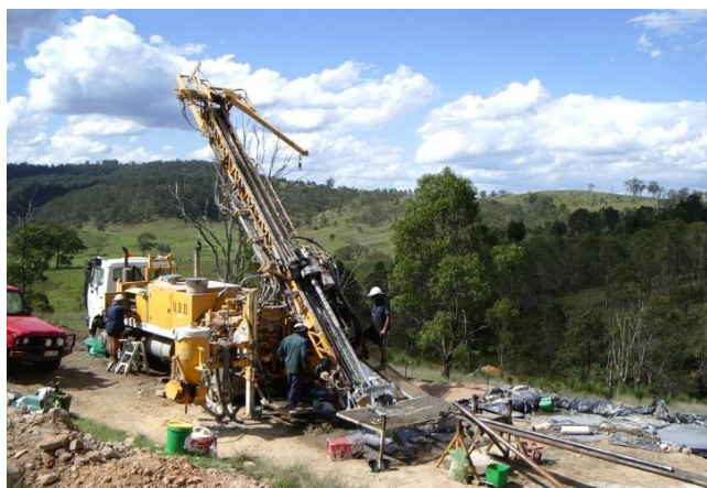
Diamond drilling (similar to water bore drilling) is one of the most advanced forms of exploration.
