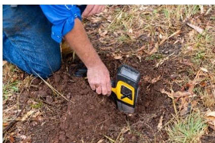
Soil sampling involves collection of approximately 1kg samples and is usually undertaken using handheld tools. Over a grid that is measured using a handheld GPS, a shovel is used to dig a shallow hole, then soil is checked with a handheld XRF. A small (1kg) sample is then collected and sent for laboratory analysis.
