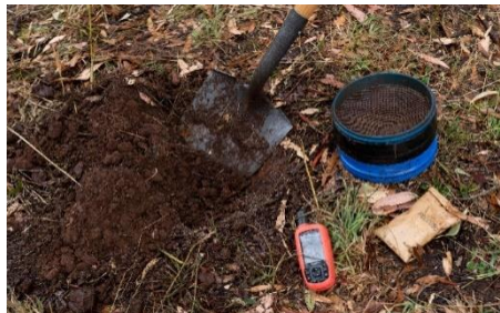
Soil sampling involves collection of approximately 1kg samples and is usually undertaken using handheld tools. Over a grid that is measured using a handheld GPS, a shovel is used to dig a shallow hole, then soil is checked with a handheld XRF. A small (1kg) sample is then collected and sent for laboratory analysis.
