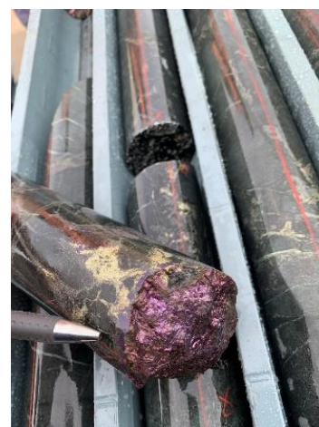
Diamond drilling can bring cores of rock to the surface so that geologists can analyse the minerals – many call it the 'truth machine' for exploration.
