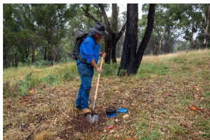
Soil sampling involves collection of approximately 1kg samples and is usually undertaken using handheld tools. Over a grid that is measured using a handheld GPS, a shovel is used to dig a shallow hole, then soil is checked with a handheld XRF. A small (1kg) sample is then collected and sent for laboratory analysis.
