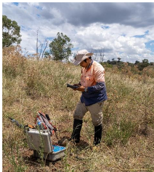
Induced polarisation surveys can be used to identify aquifers and metallic minerals.
